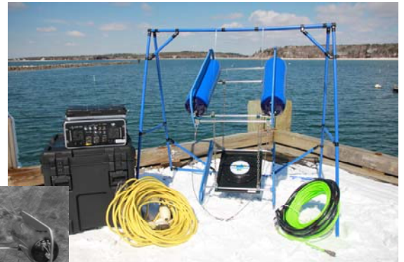
Complete Single-Source Bubble Gun System (shown with source vehicle suspended on display frame)
