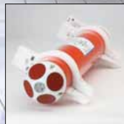
DVS 750m with optional OEM Thermistor (left), and without (right).
