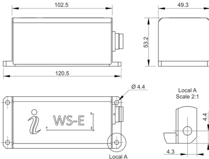
**Wave Sensor (WS-PD) Mechanical Interface Drawings**
