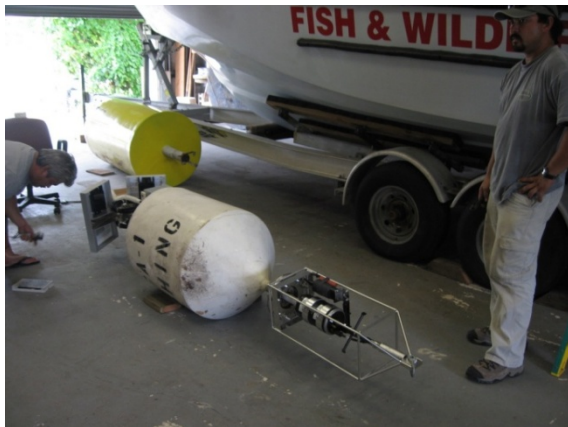
Buoy-Mounted 2D-ACM Current Meter being readied for deployment
